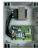
230 V control panel with 433.92 Mhz built-in receiver
