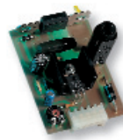
Battery charger card for VE.250/I, VE.500/I - VE.650/I - DA.24A
