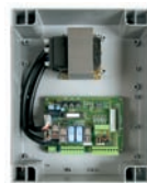
230 V control panel with 433.92 receiver
